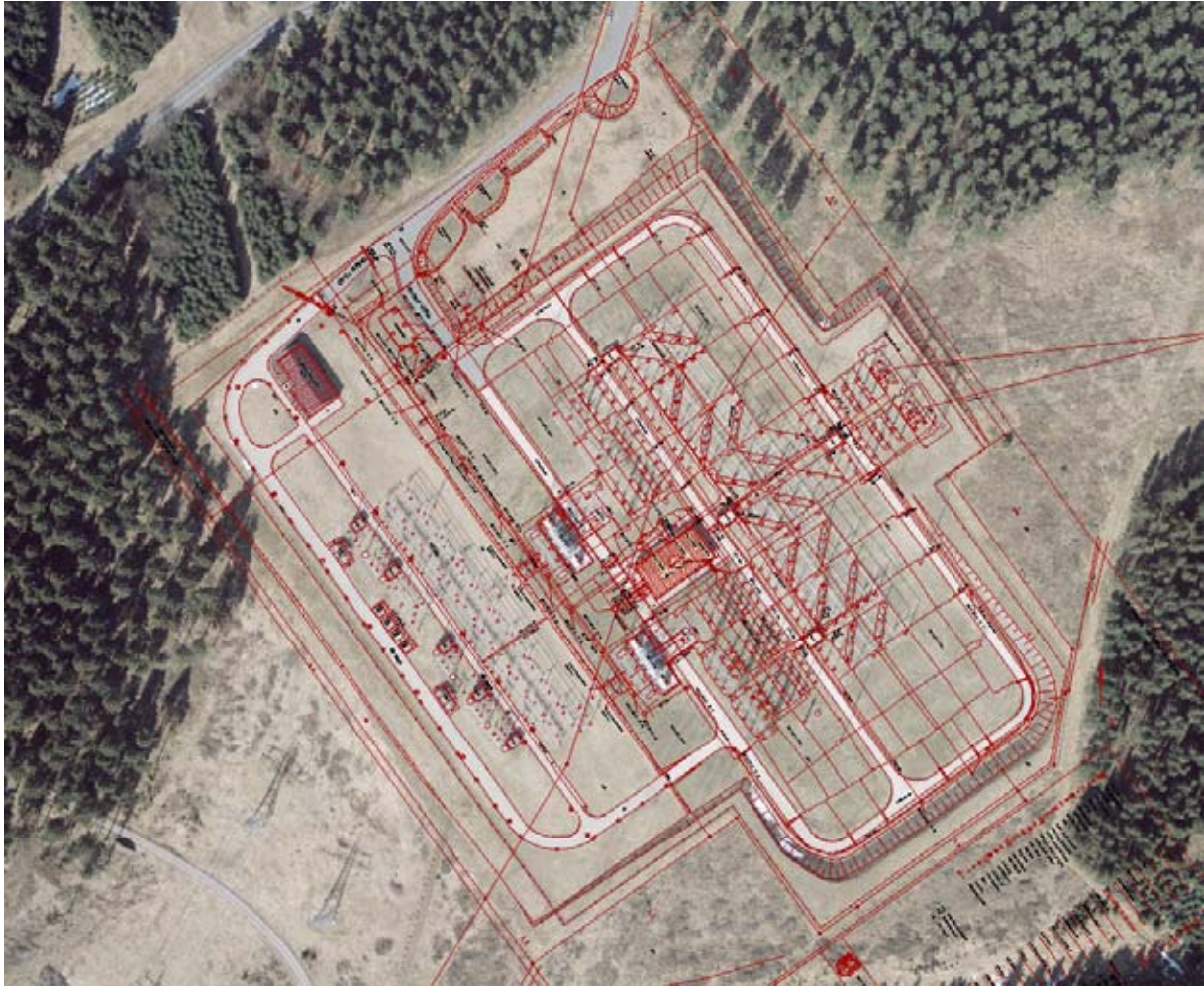
Fig. 6: Power supply installation. The image has been rectified based on direct sensor orientation with DGPS and inertial navigation system (INS).
