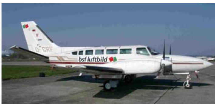
Fig. 3 (top): One of the aircraft of the BSF Luftbild GmbH: The Cessna 404 with two camera openings to operate double sensors.
