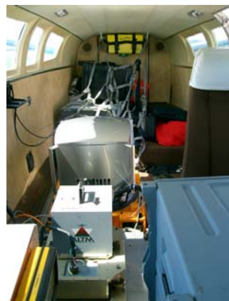
Fig. 3 (top): One of the aircraft of the BSF Luftbild GmbH: The Cessna 404 with two camera openings to operate double sensors.
